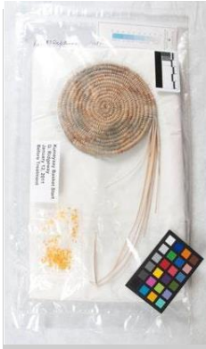
Image 5: The basket starts in a polyethylene bag. The blue strip in the upper left corner measures relative humidity. The yellow beads (silica gel) remove moisture.
