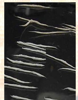
Image 4: Japanese tissue paper, rolled into "stitch-shaped" Frankenstein mends, prior to application
